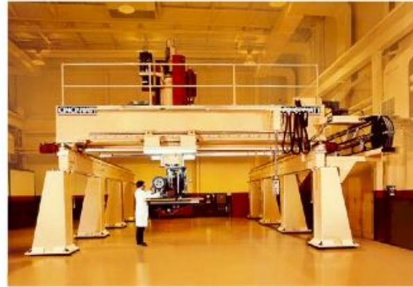
Fig 1.0 Tape Layer Configuration and Axis of Movement
