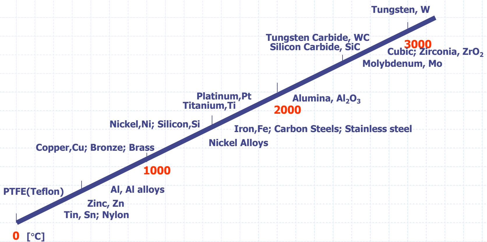
Melt temperature for crystalline metals and ceramics and semi crystalline thermoplastic polymers
