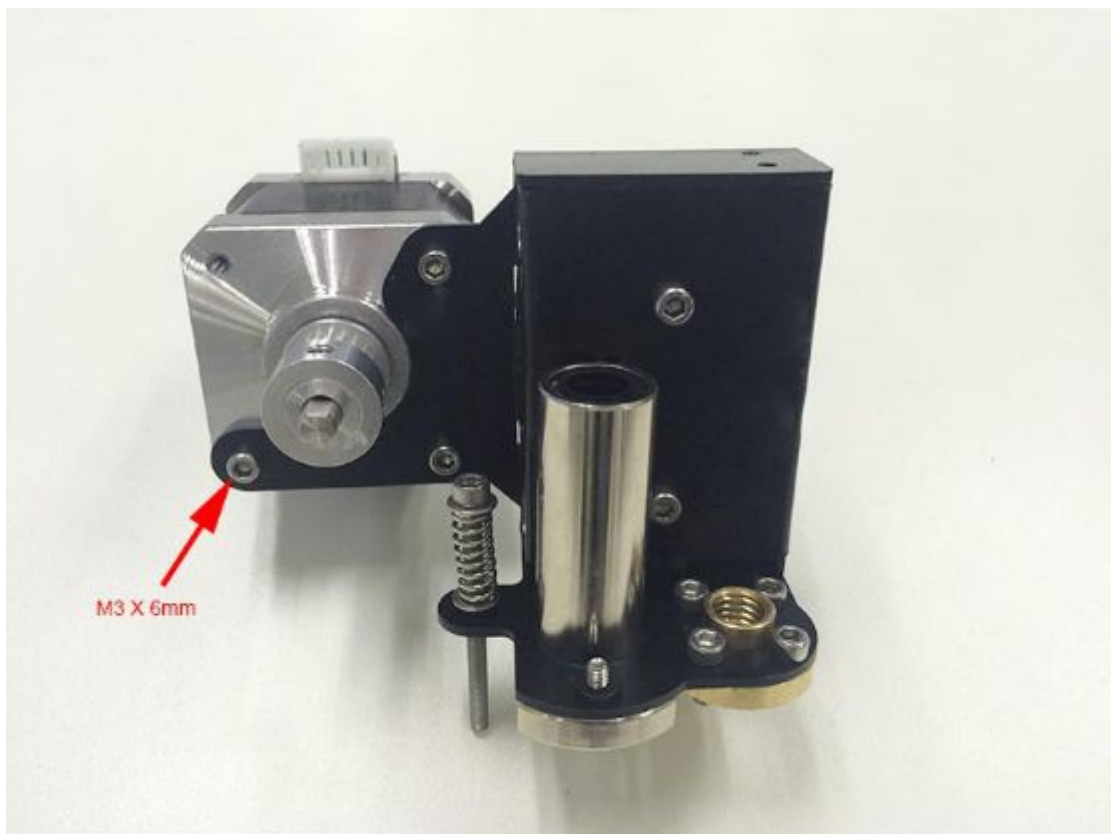
Step 2. Mount the stepper motor on the motor end with 3 M3 x 6 mm screw.
