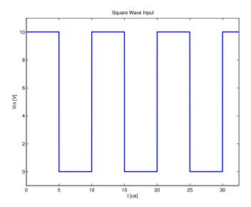
Any square wave can be represented by a Fourier series. To keep things simple, rather than find the entire Fourier series, we'll just decompose it into two parts: the DC component, and the square wave excluding the DC component.
