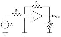
(b) Now just for (b), let  $R_1=100\,\Omega,\,R_2=2\,\mathrm{k}\Omega,\,R_3=1\,\mathrm{k}\Omega,\,i_L=10\,\mathrm{mA}.$  Calculate  $V_{out}$  and  $V_{in}$ .
