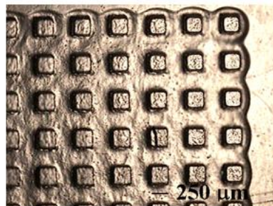
i) Micro well embossing insert (top view) j) HDPE embossed micro wells
