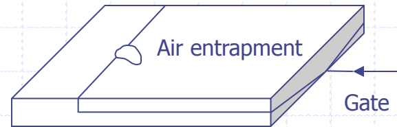
Edge gate: warp free, air entrapment
