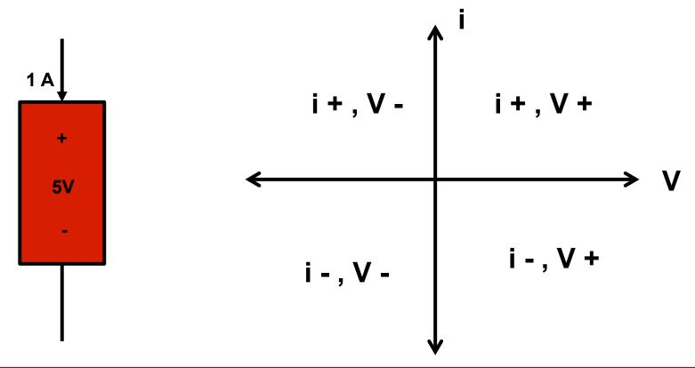
• Note that the energy is dissipated by the device in quadrants 1 and 3, and power is generated by the device in quadrants 2 and 4.
