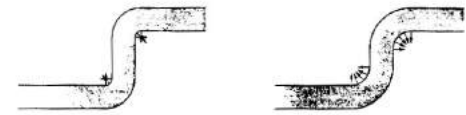
Figure 7.2.24 Identifying hot spots in castings by using outward projecting arrows of length half the casting thickness. Where arrows overlap, hot spots may develop. (Courtesy of Meehanite Metal Corp.)
