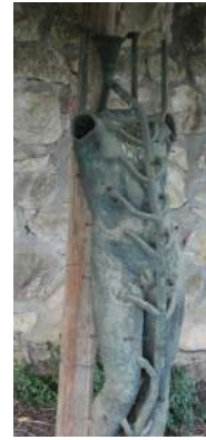
Etruscan casting with runners circa 500 BCE
